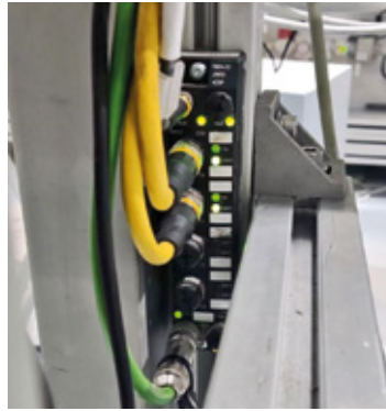
Turck's compact TBEN-S2 RFID interface ensures fast and reliable data transmission
