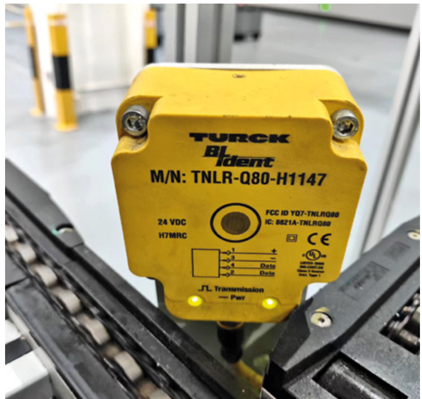
Thanks to its large range, Turck's robust Q80 HF read/write head enables reliable RFID detection even if the position of the tags varies
