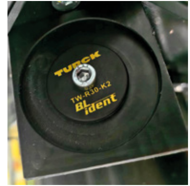
With 10 billion write operations, the TW-R30-K2 also guarantees very good readability in the long term
