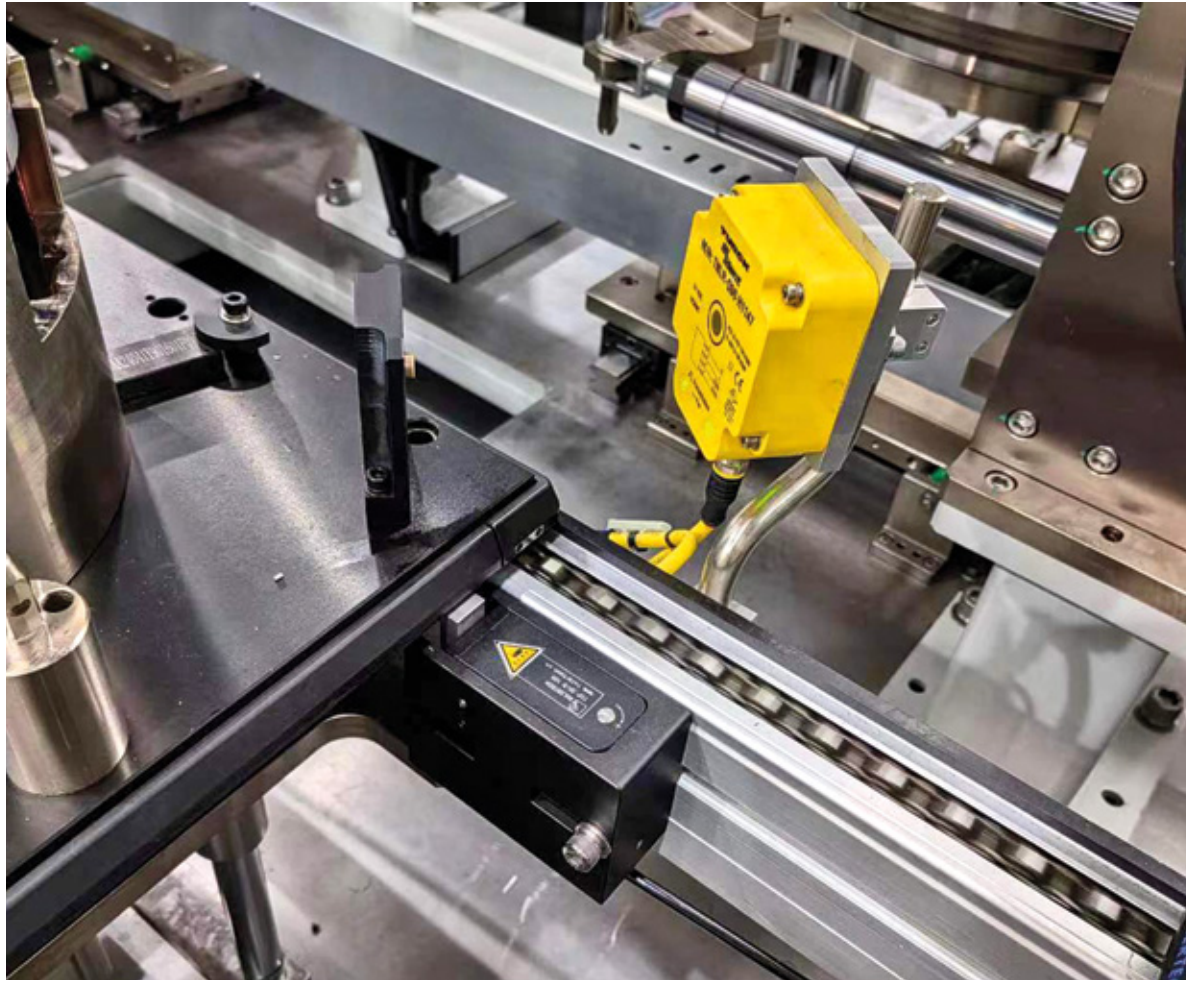
RFID tags on the workpiece carriers store production data and enable unique identification of the material on the carrier plate
