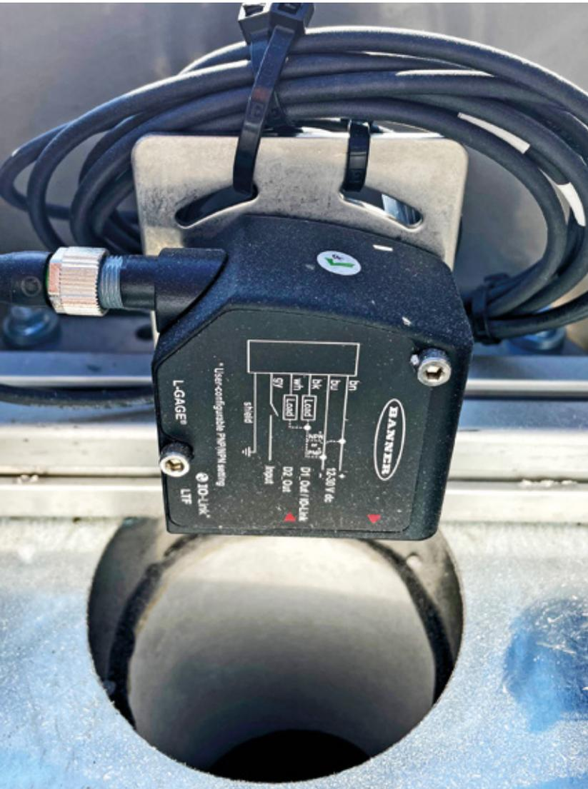
The robust LTF12 laser sensor with an IO-Link output has a range of up to 12 meter with a resolution of 0.3 to 3 millimeter
