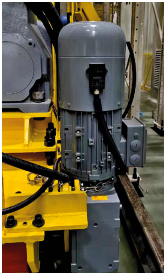
Three CMVT sensors are used for each stacker crane, one for each motor
