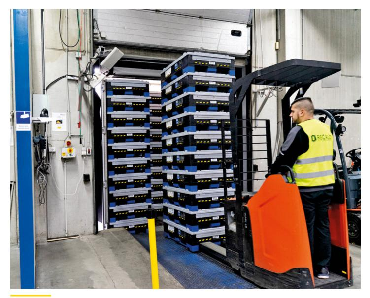
The stacked RTIs are fully logged when the forklift passes through the gate when the truck is loaded
